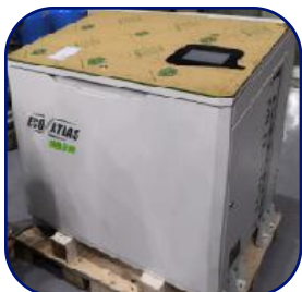
18U浸没式液冷服务器机柜 18U immersed liquid cooling server cabinet
